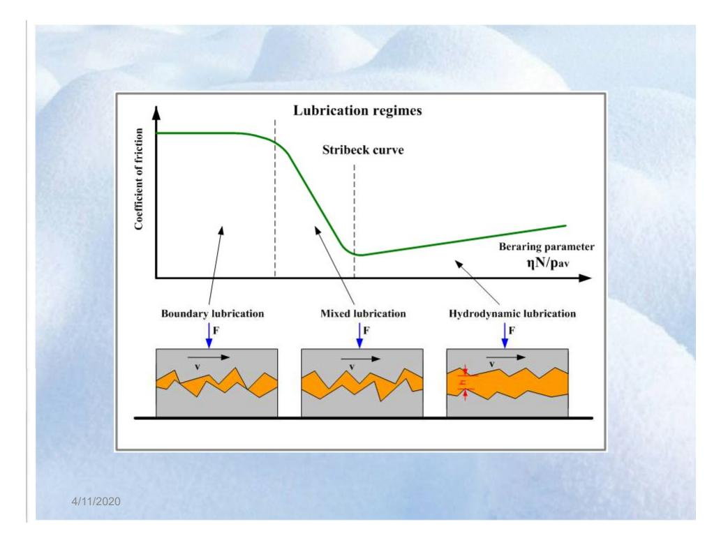
The three lubrication regimes are clearly distinguished in the Striebeck curve (see the figure above), which demonstrates the relationship between the coefficient of friction and the bearing parameter  $\eta^*N/p_{av}$  ( $\eta$  - dynamic viscosity of the lubricant, N - rotation speed,  $p_{av}$  - average bearing pressure).
