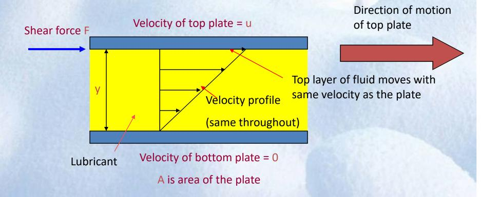
•There is no pressure buildup in the fluid due to relative motion
