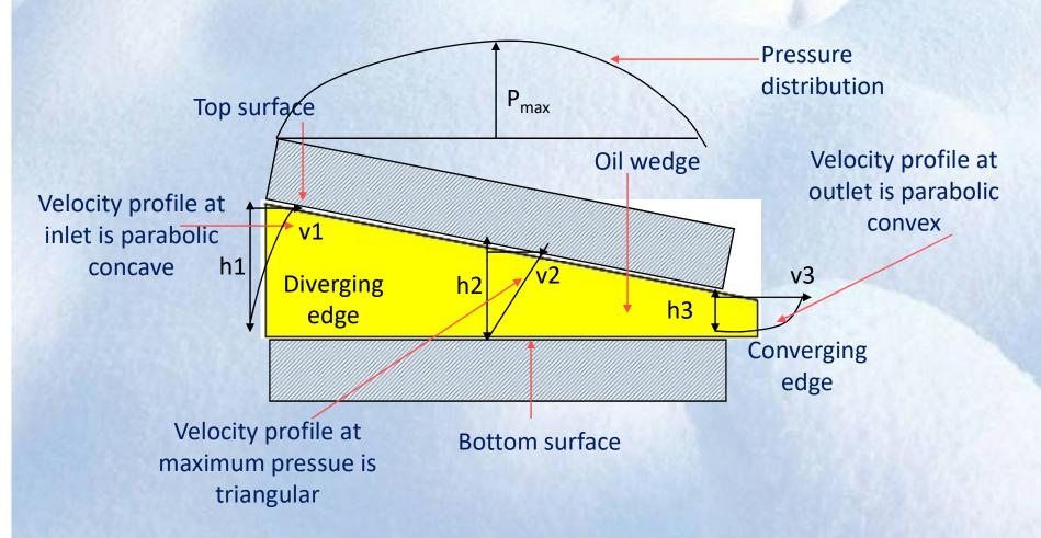
Volume rate of flow is same throughout the path, therefore as height of film decreases, the velocity has to increase (v3>v2>v1)
