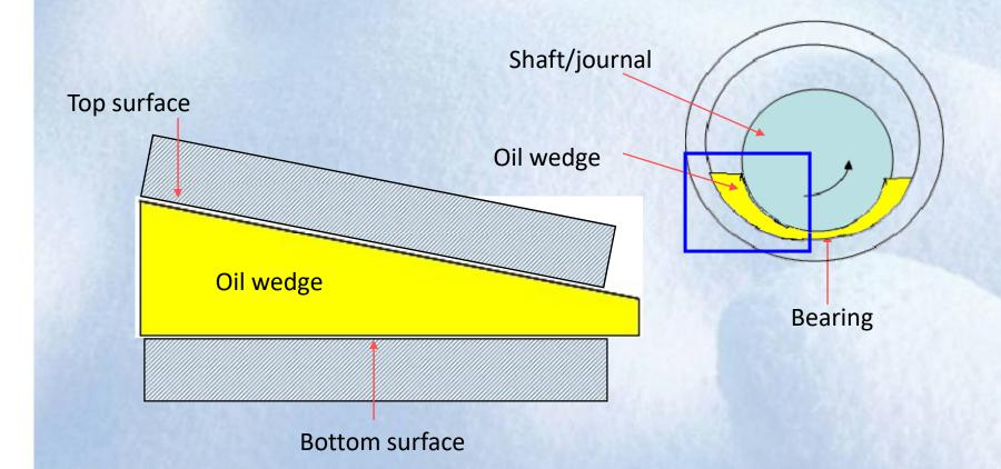
Oil wedge forms between shaft/journal and bearing due to them not being concentric
